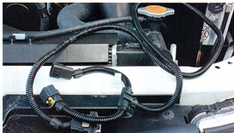
Tuning module wiring sits between the vehicle's standard wiring and the fuel injection connector plug on a common rail diesel engine
